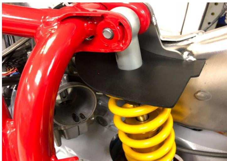
A good idea also is this 'home-made' small extra flap that bolts on where the air intake flap is cover is. It approx. 20mm in width and also helps to stop water splashing UP into the filter box.
